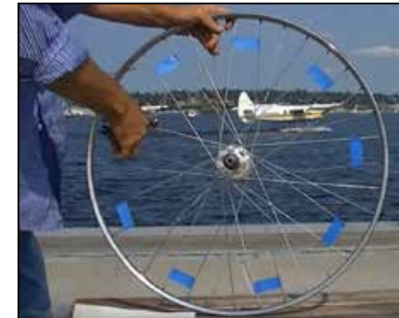
Mark with tape the spokes you wish to keep and remove other spokes.
