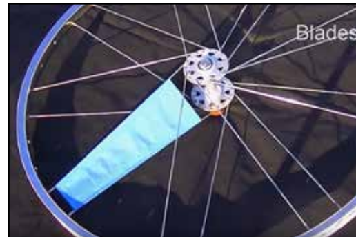
Using duct tape or shrink wrap plastic create the blades as shown.
