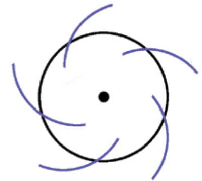
The barrel is divided into five panels - you will need a protractor to get the right spacing of the panels - 360 degrees divided by 5 = 72 degrees.
