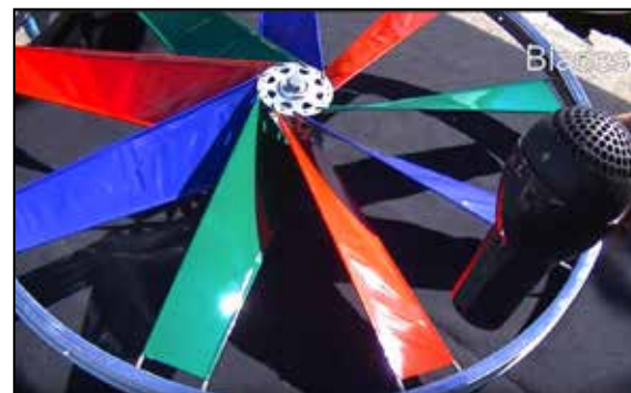
You will need a hair dryer to heat the shrink wrap into place
