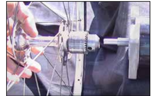
Insert a bolt through the axle hole and lock in place then fix a drill chuck to complete the windmill element.
